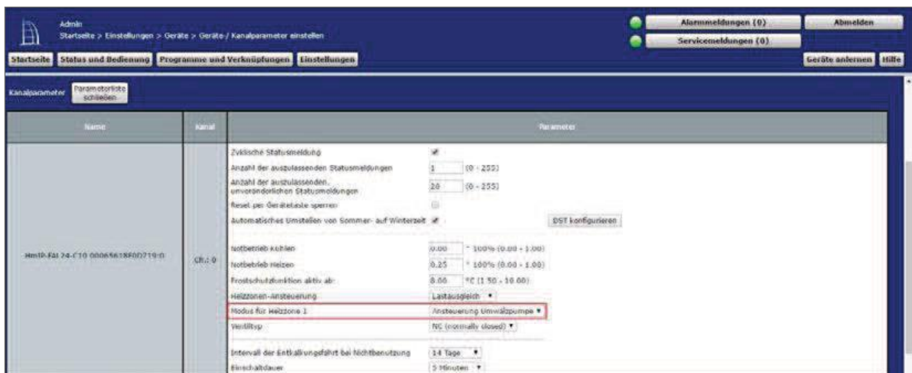
Figure 239: Configuration Channel parameter Floor Heating Actuator
