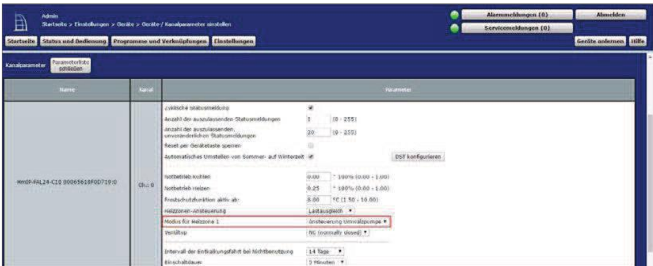
Figure 213: Configuration Floor Heating Actuator
