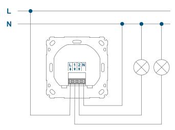
A neutral conductor is required for installation
